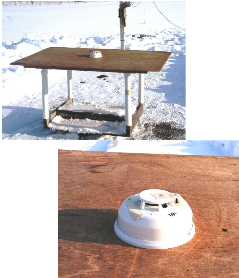
Figure 4: Radiated Emissions Test Setup Photograph(s).
