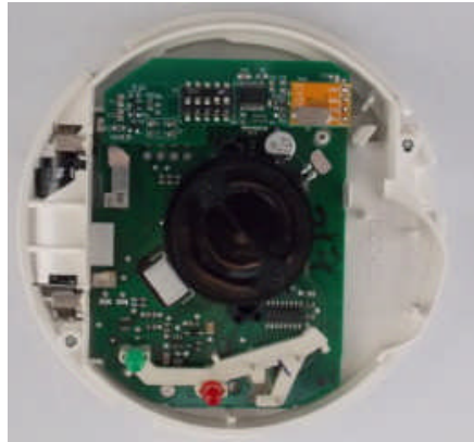
Control PCB Rear
