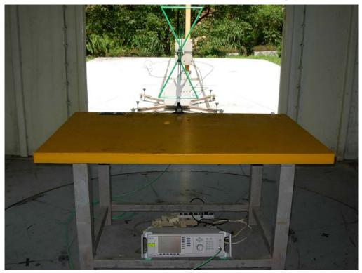
Test Mode : Mode 1: Receive Description : Back View of Radiated Emission Test Setup(Bi-Log)
