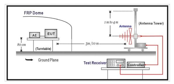
Above 1GHz Test Setup:
