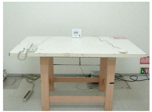
Test Mode: Mode 1: ReceiveDescription: Back View of Conducted Emission Test Setup
