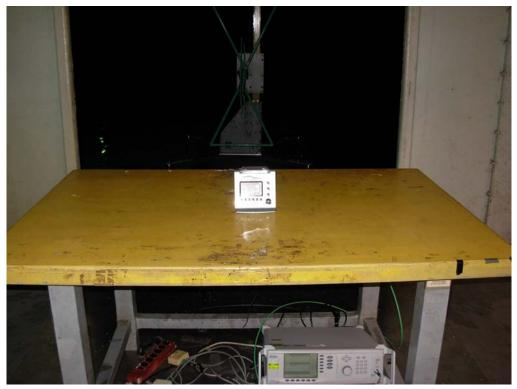
Test Mode : Mode 1: Receive Description : Back View of Radiated Emission for Superregenerative Receiver Test Setup
