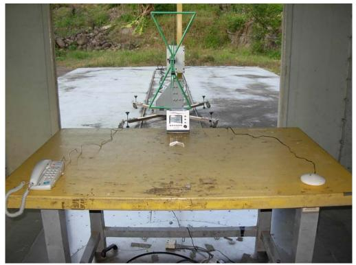
Test Mode: Mode 1: ReceiveDescription: Back View of Radiated Emission Test Setup
