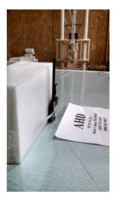
Harmonics Test with Horn Antenna for over 1 GHz – Flat Orientation
