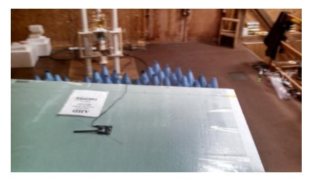
Harmonics Test with Horn Antenna for over 1 GHz – Side Orientation
