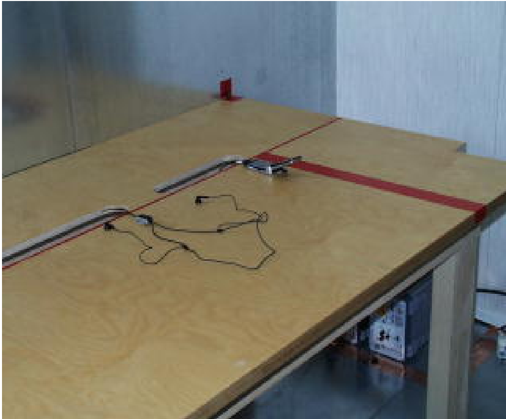
Picture 1 AC powerline conducted emission measurement
