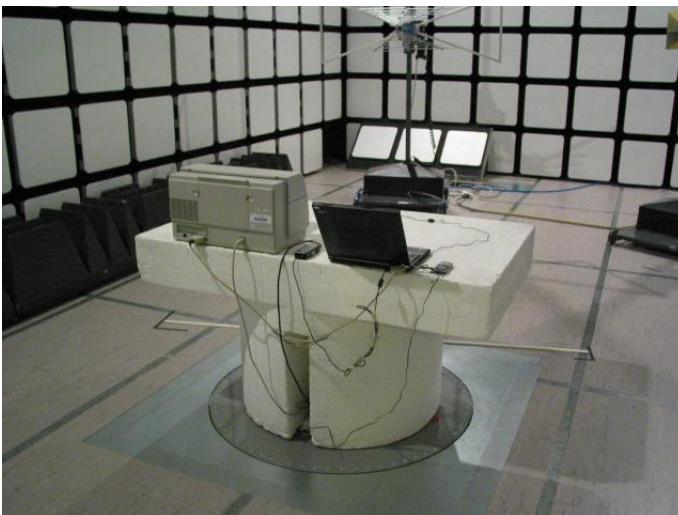
Picture 2. FCC Part 15B Radiated emissions
