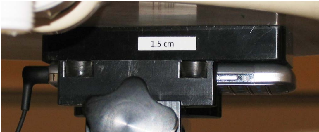
Photo of the device positioned for Body SAR measurement. The spacer was removed for the tests.
