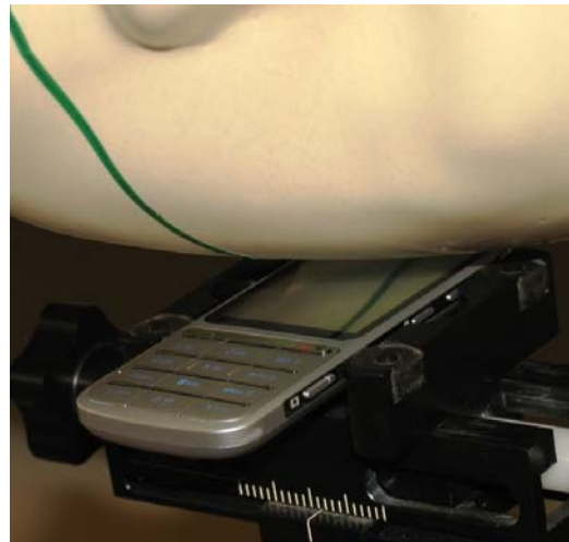
Photo of the device in “tilt” position
