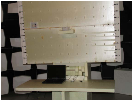
Picture 2. FCC Part 15B Radiated emissions
