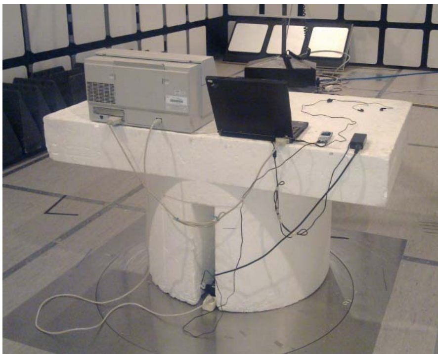
Picture 2. FCC Part 15B Radiated emissions
