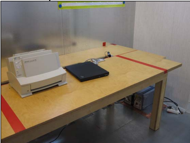
Picture 4 AC powerline conducted emission measurement 15B
