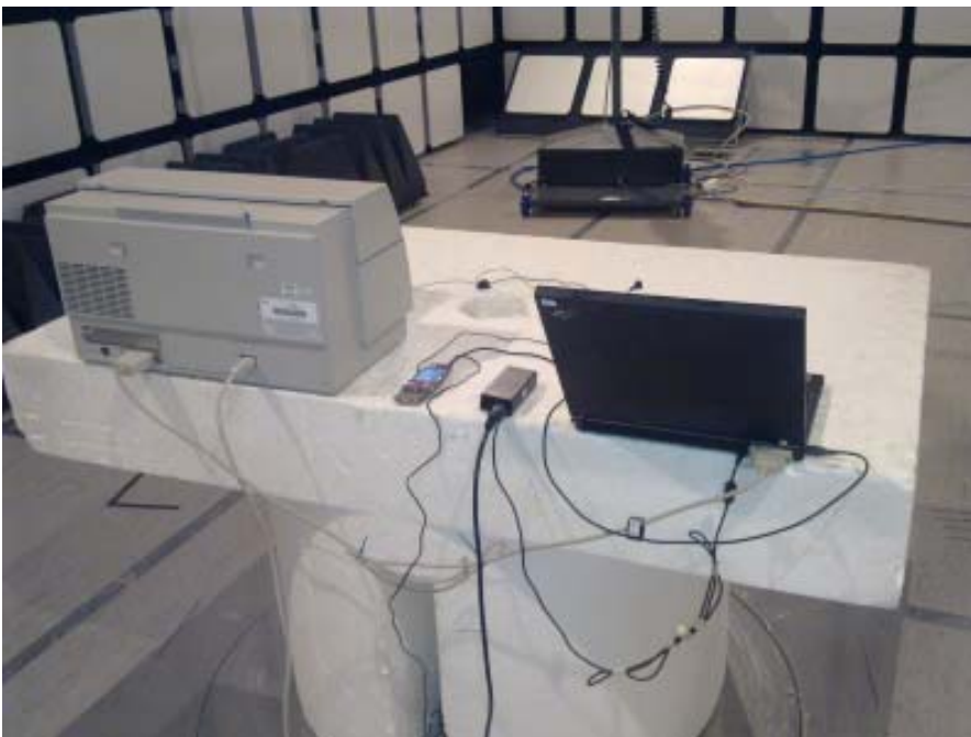
Picture 2. FCC Part 15B Radiated emissions
