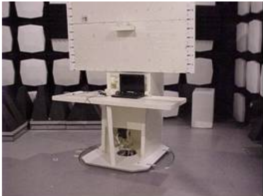
Picture 2. FCC Part 15B Radiated emissions
