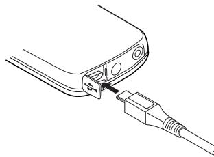
Open the cover of the USB connector, and connect the USB cable to the device.
