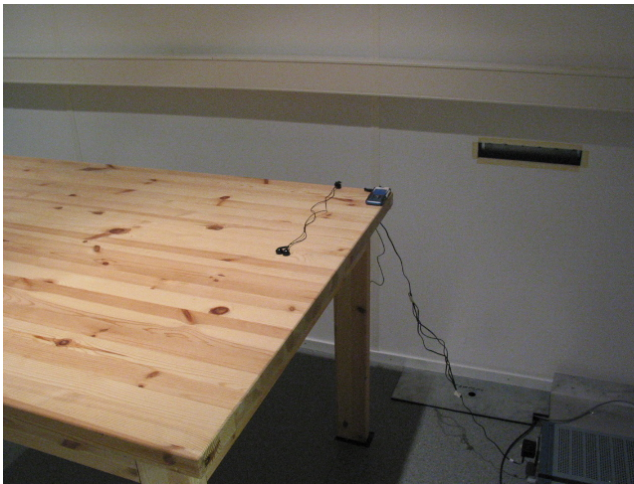
Picture 3 AC powerline conducted emission measurement Bluetooth TX
