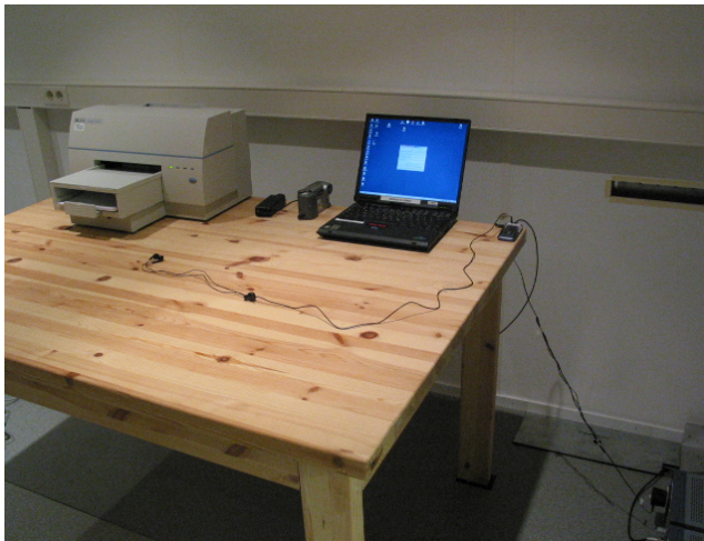
Picture 4 AC powerline conducted emission measurement GSM RX + Computer peripherals
