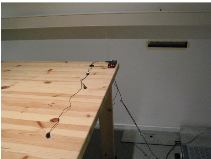
Picture 4 AC powerline conducted emission measurement GSM RX + MP3 player on / Bluetooth TX
