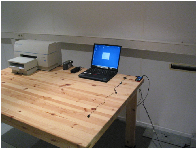
Picture 5 AC powerline conducted emission measurement GSM RX / Bluetooth TX + Computer peripherals
