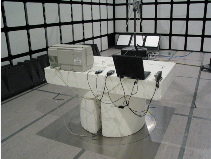
Picture 1 Radiated emission measurement GSM RX / Bluetooth TX + Computer peripherals
