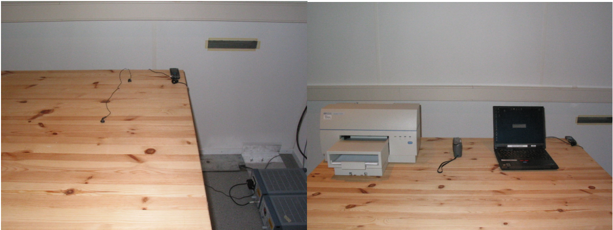
Picture 3 AC powerline conducted emission measurement GSM RX / Bluetooth TX
