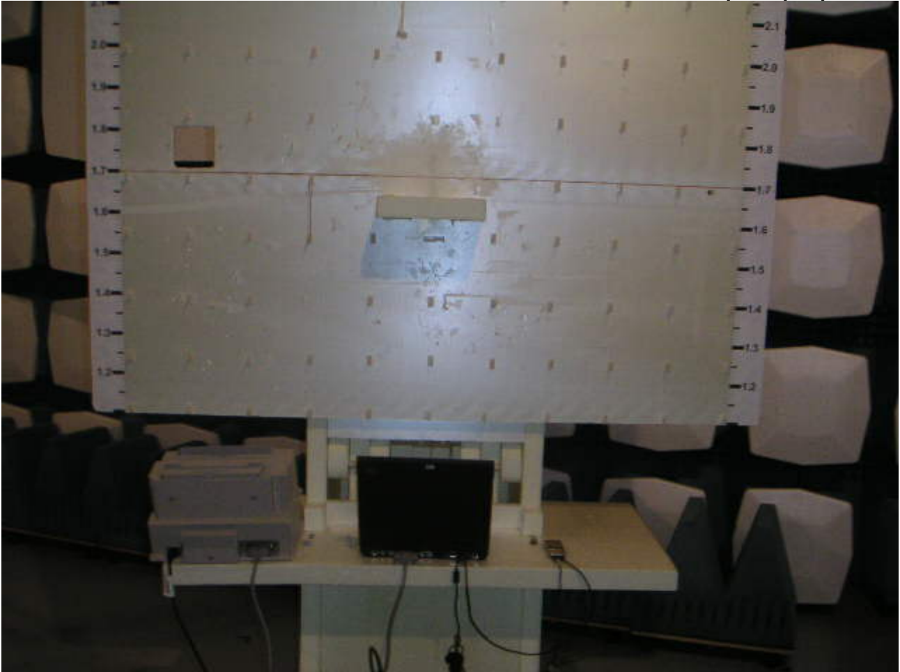
Picture 2 Radiated emission measurement GSM 1900 RX and BT TX + Computer peripherals
