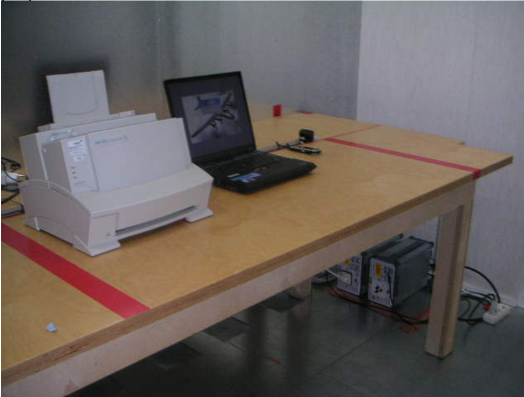
Picture 4 AC powerline conducted emission measurement WLAN TX + Computer peripherals
