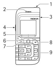
The 5-way joystick is also used to move the cursor up and down, and left and right when writing text, using the calendar, and in some game applications. Pressing the joystick also functions as the middle selection key, and pressing it briefly selects the function shown on the display above the joystick.
