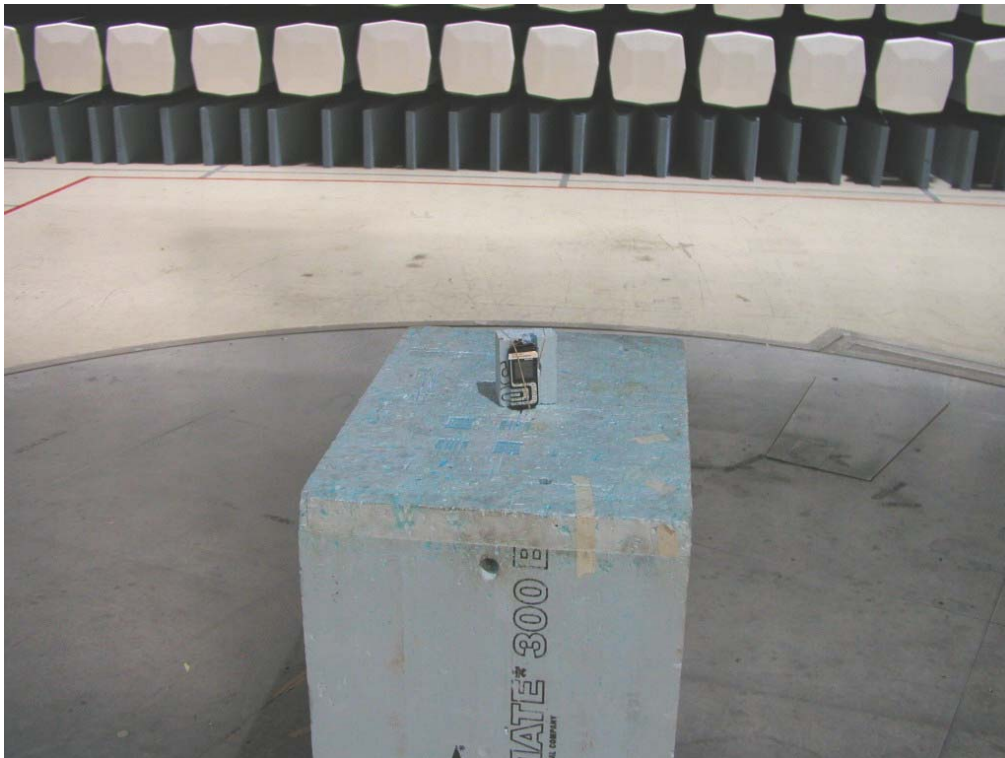
Photograph 1. Radiated RF output power and spurious radiated emissions test setup
