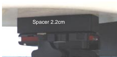
Photo of the device positioned for Body SAR measurement. The spacer was removed for the tests.
