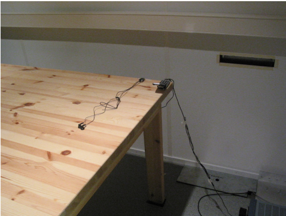
Picture 3 AC powerline conducted emission measurement
