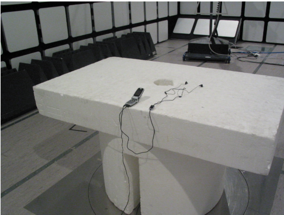
Picture 2 Radiated emission measurement
