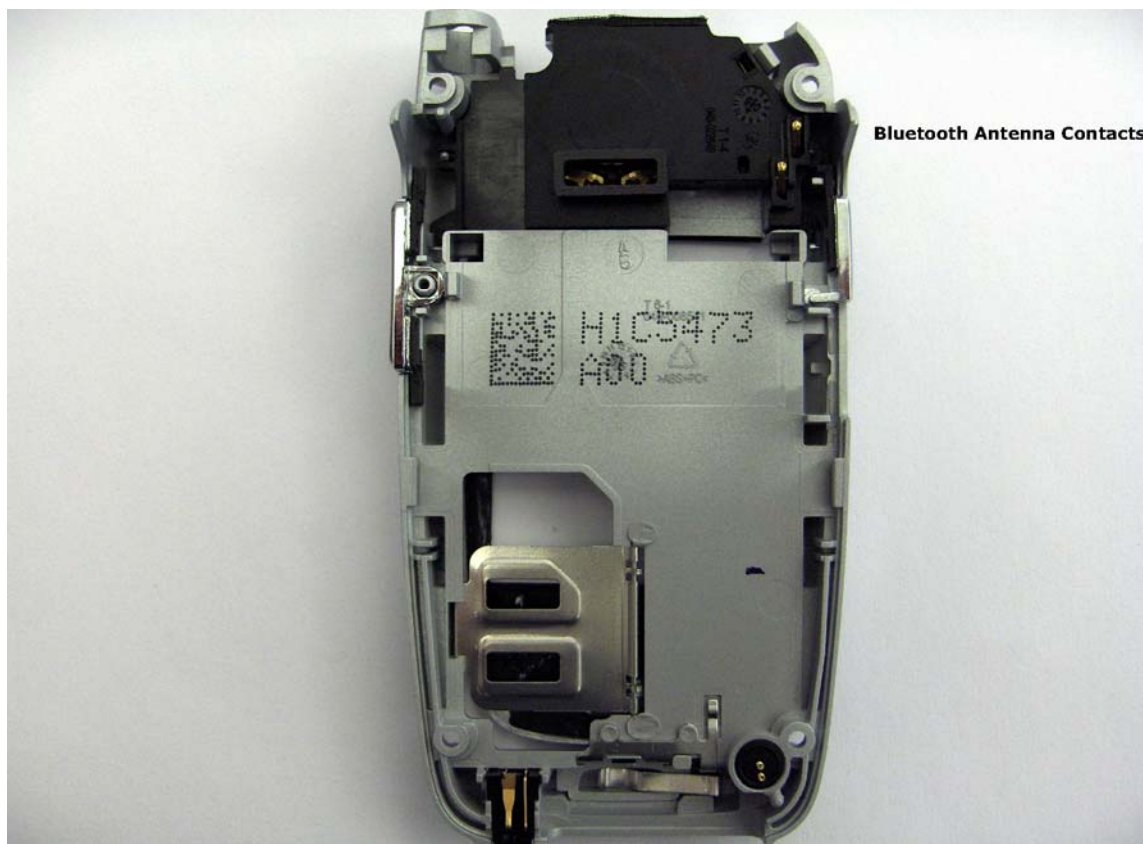
Cover showing the contact points for Bluetooth antenna
