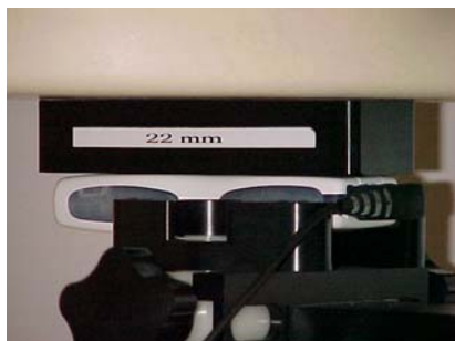
Photo of the device positioned for Body SAR measurement. The spacer was removed for the tests.
