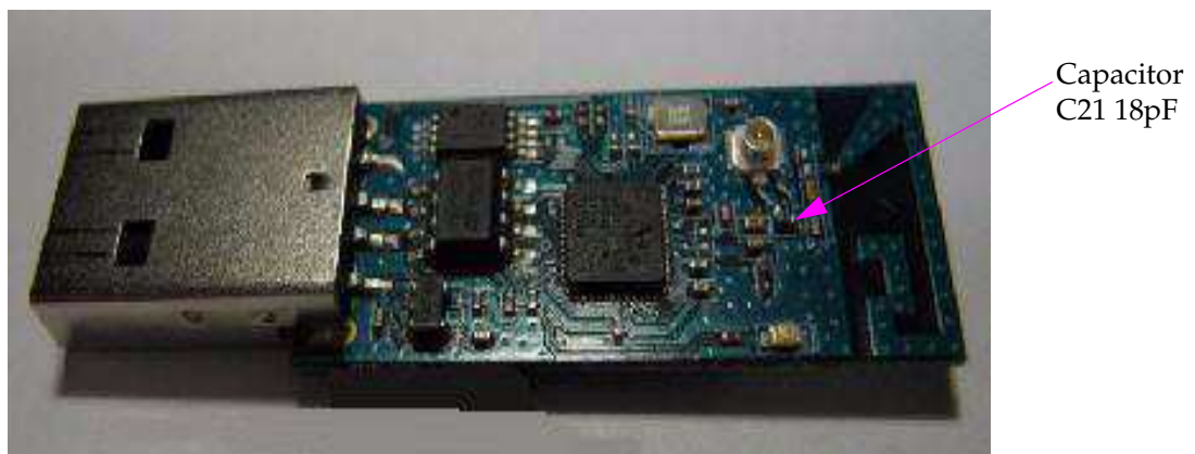
Figure 1-9. Location of the Capacitor on the Bluetooth Adapter
