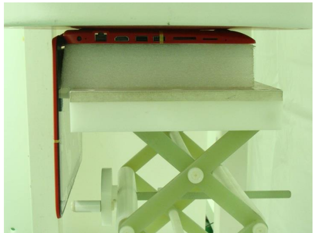
Bottom of Laptop, Test Separation 0 cm (NB Mode_WNC)
