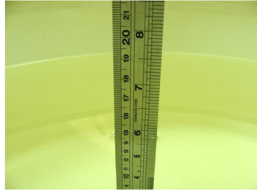
Fig 6.2 Photo of Liquid Height for Body SAR
