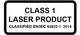
This device is classified as a Class 1 laser product per *EN/IEC 60825-1:2014*. This device complies with FDA performance standards for laser products except for conformance with *IEC 60825-1 Ed. 3*, as described in *Laser Notice No. 56*, dated May 8, 2019.
