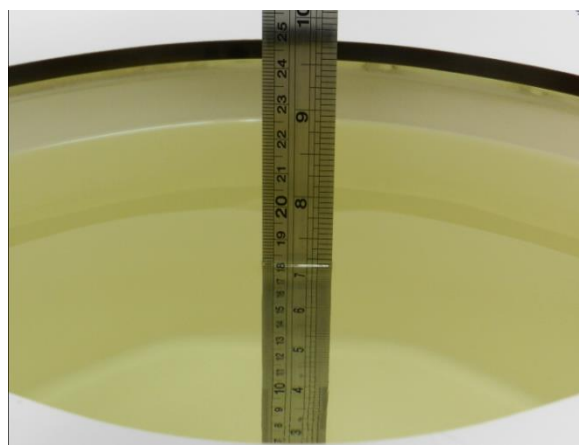
Fig 10.2 Photo of Liquid Height for Body SAR
