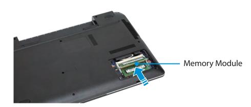
4 Push the memory module down so that it is completely fixed. If the memory does not fit easily, push the memory module down while pulling the memory module latches outward.
