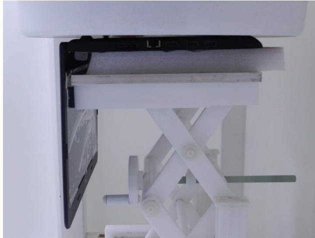
Bottom of Laptop, Test Separation 0 cm
