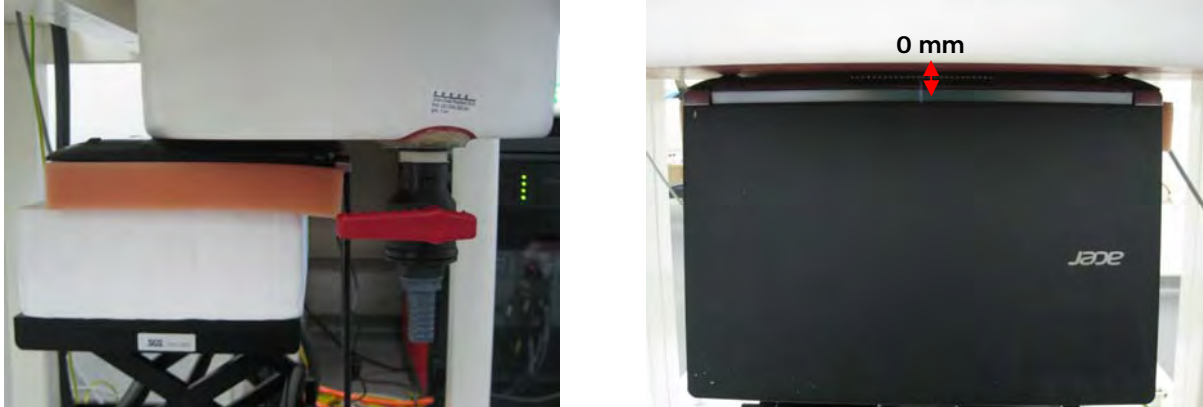
Fig.3 EUT Lap-held mode to flat phantom
