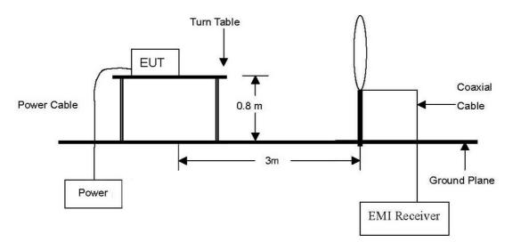
The diagram below shows the test setup that is utilized to make the measurements for emission from 30 Mz to 1 GHz Emissions.
