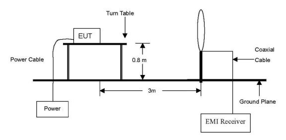
The diagram below shows the test setup that is utilized to make the measurements for emission from 30 Mb to 1 GHz Emissions.
