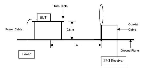
The diagram below shows the test setup that is utilized to make the measurements for emission from 30 Mb to 1 GHz Emissions.
