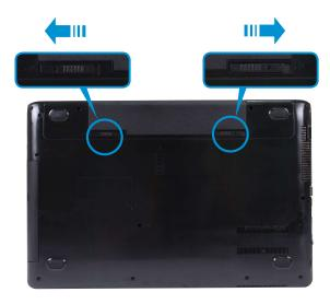
To install the battery again, slide the battery into the system. The battery latches move inwards and fix the battery automatically.
