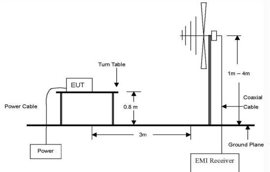
The diagram below shows the test setup that is utilized to make the measurements for emission .The spurious emissions were investigated form 1 Glz to the 10th harmonic of the highest fundamental frequency or 40 Glz, whichever is lower.
