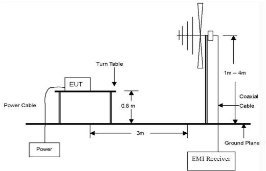
The diagram below shows the test setup that is utilized to make the measurements for emission. The spurious emissions were investigated form 1  $Gl_2$  to the 10th harmonic of the highest fundamental frequency or 40  $Gl_2$ , whichever is lower.
