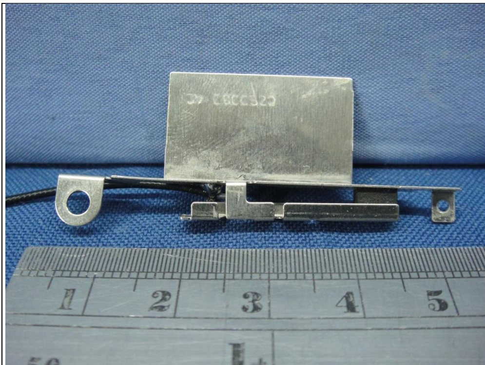
Antenna (Brand : WNC, Model : 81-EBJ15.005<3.62dBi>)
