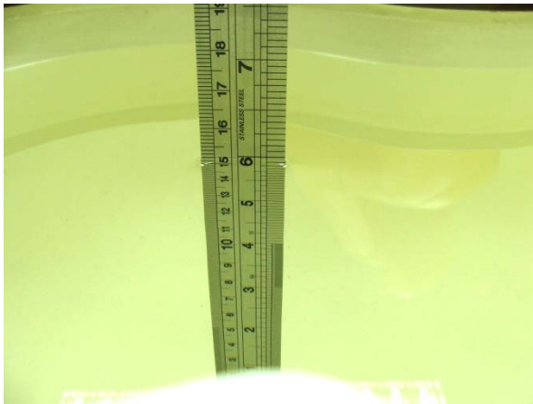
Fig 6.1 Photo of Liquid Height for Head SAR
