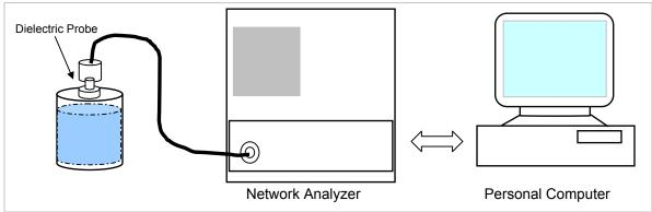
Set-up for liquid parameters check
