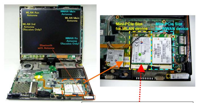
The certification label is stuck on the top side of the applying transmitter device, and the FCC ID is visible when the palm rest assembly is removed.
