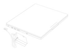
Attach the cord from the power adapter as indicated. Please do not use other, nonapproved power adapters. The battery is not fully charged when your Chromebook Pixel arrives, and will charge once the power adapter is connected. You will know that charging is complete when the power input light changes from yellow to green.
