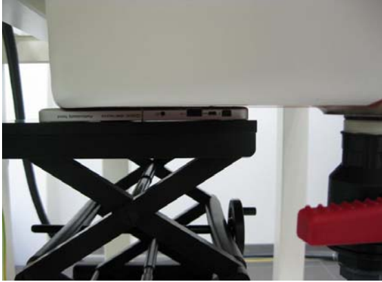
Fig.3 EUT Lap held mode to flat phantom
