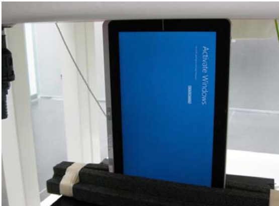
Fig.4 EUT Secondary Portrait mode to flat phantom
