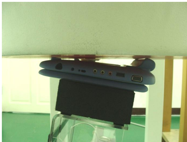
Fig 9.5 Bottom of Tablet Touching with 0 cm Air Gap (DUT with Battery 2)
