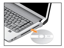
To eject a disc from the drive, gently touch the eject control. The control will flash to confirm a few seconds before ejecting the disc.
