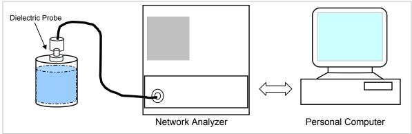
Set-up for liquid parameters check
