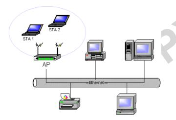
To connect to an access point network, configure the profile for access point mode.
